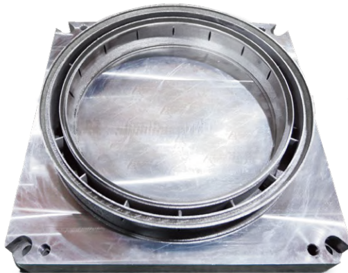
Engine leaf ring structure 316L stainless steel \Phi 400 \times 60 \text{ mm}^3
